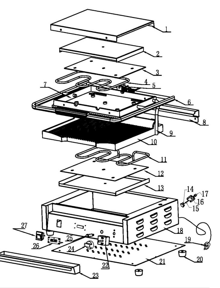
Exploded diagram and spare parts list
